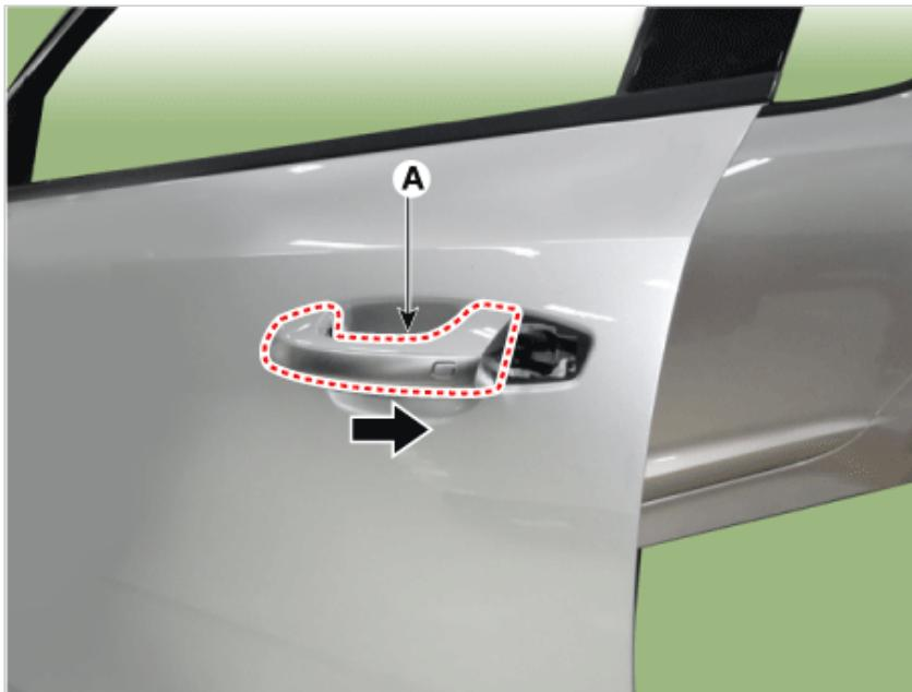
4. Disconnect the front door outside handle connector (A).
